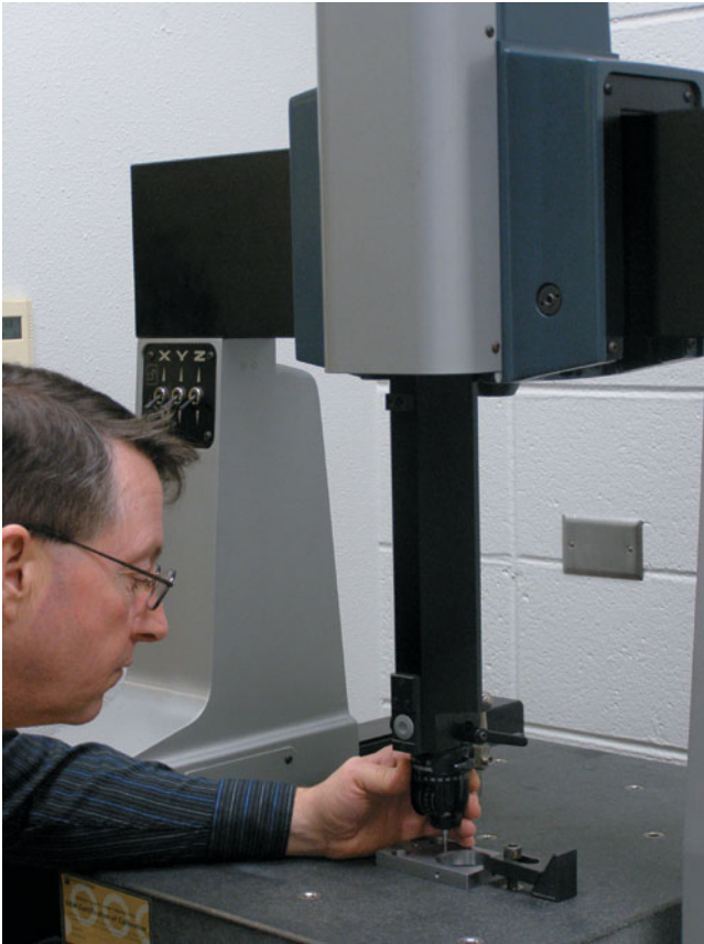
Figure A-3 Quality control technician using a CMM to inspect a part (Courtesy of Fox Valley Technical College).
